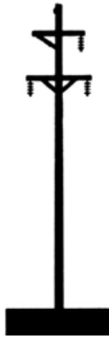
SPT-2 Distribution to 138kV
