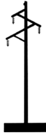
SPT-3 Distribution to 138kV
